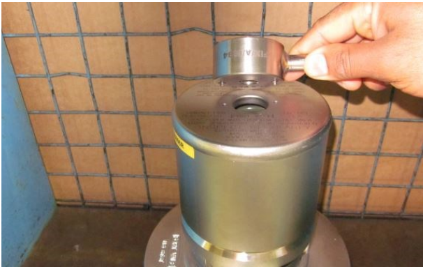
Step 9. Select the cap tightening tool, part number FIX/A/0034. Engage the two pins on the cap tightening tool into the two blind holes of the top cap.
