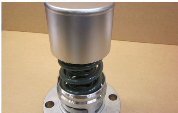
Step 34. To complete the assembly procedure, move the valve to a bench press with a minimum 1 tonne load. WARNING: Relief valves are spring-loaded and can cause serious personal injury. Obey all the instructions and wear eye protection during this procedure.
