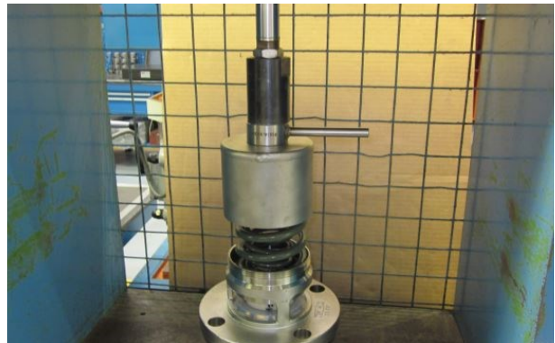
Step 12. When the valve and the cap are disassembled, unlock the press and gradually retract the press to release the spring load. WARNING: Be careful when you retract the press. Make sure that the spring is fully decompressed before you remove the ram.
