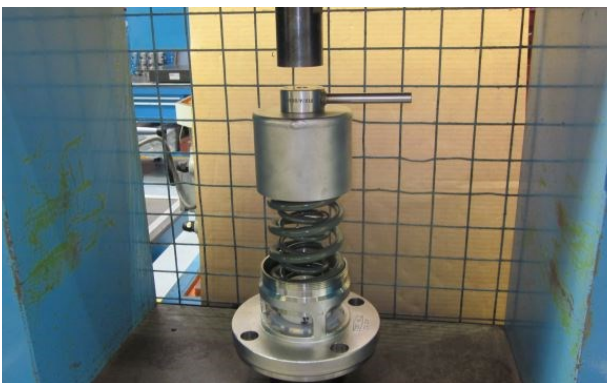
Step 39. Make sure that the cap tightening tool is located correctly on the top cap. Make sure that the valve assembly is centrally aligned to the ram.
