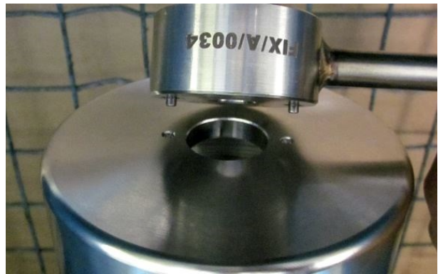
Step 38. Select the cap tightening tool, part number FIX/A/0034. Locate the two pins on the cap tightening tool into the two blind holes of the top cap.
