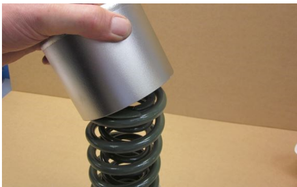
Step 33. Install the top cap onto the springs. Make sure that the springs engage in the groove inside the top cap.
