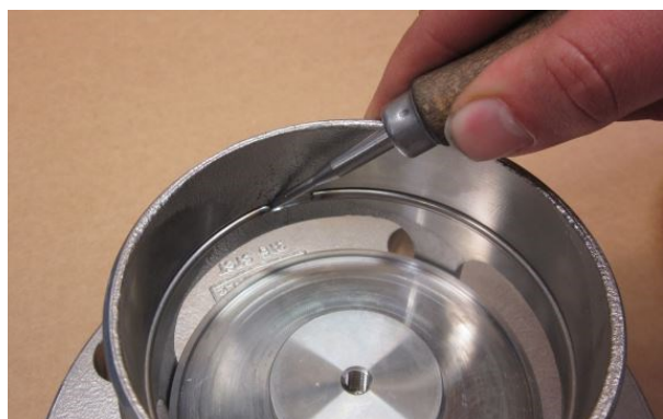
Step 18. Use a sharp-edged tool to detach the retaining ring clip.
