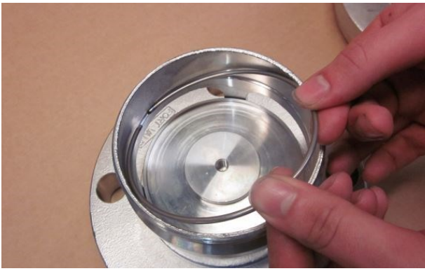
Step 19. Remove the retaining ring clip.
