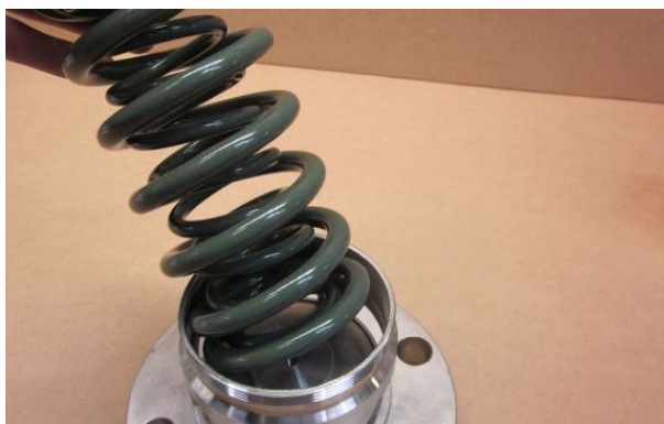
Step 30 Examine the springs for signs of damage or corrosion. If satisfactory, install the springs. If there is damage, contact Fort Vale.
