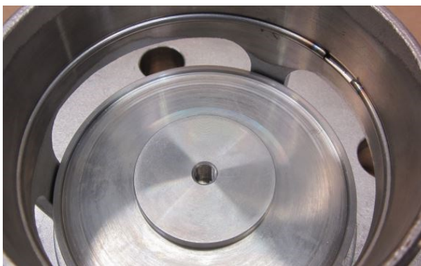
Step 29. The retaining ring clip correctly installed in the groove.
