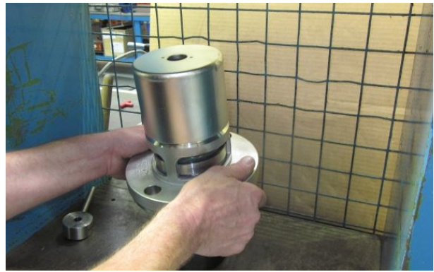
Step 8. Install the valve onto the nylon lifting spacer. Make sure that the valve is central on the spacer.
