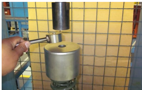
Step 14. Remove the cap tightening tool.
