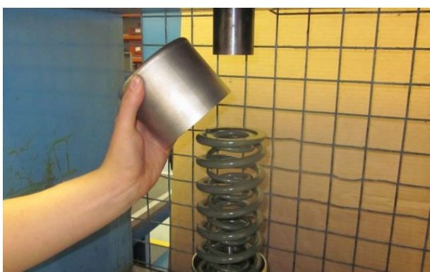
Step 15. Remove the top cap. Examine the top cap for signs of damage or wear. If there is damage, contact Fort Vale.
