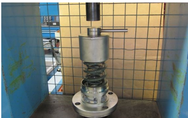
Step 13. When the spring is fully decompressed, retract the ram fully.
