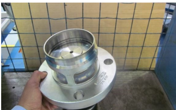
Step 17. Remove the valve body and pressure plate from the press and put it onto a work bench.
