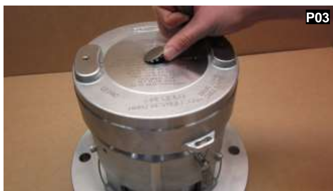
Remove the stainless steel plug.
