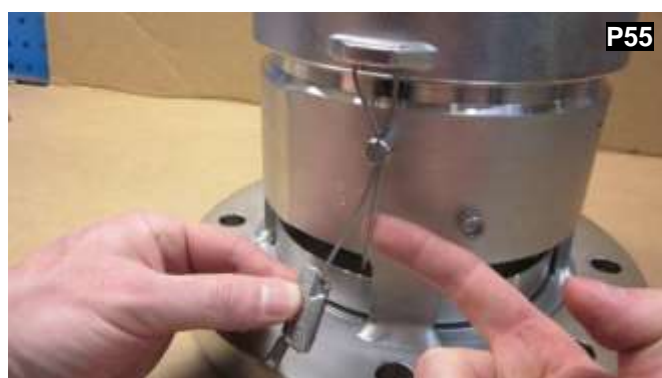
Attach the securing cable by feeding the wire through the cable nipple (As shown).
