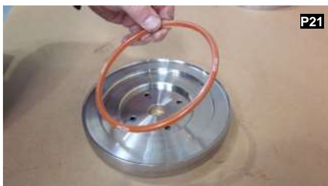
Remove the o ring. It is always recommended to change the o ring once the valve has been in service.
