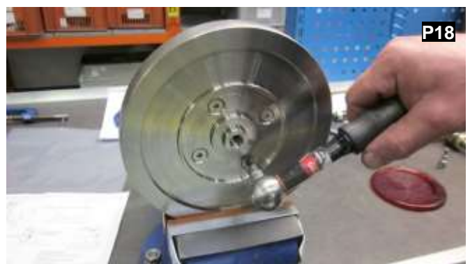
Grip the pressure plate in a soft jaws vice and loosen the bolts using a 5/32" torque wrench.
