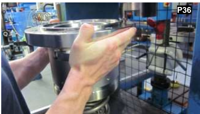
Place the main body over the pressure plate and spring.
