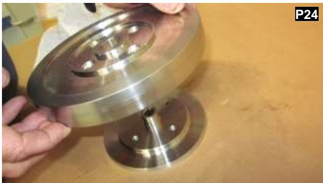
Check the inner pressure plate for any damage. If the inner pressure plate is satisfactory, place the outer pressure plate over the inner pressure plate.
