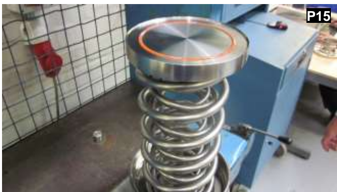
Remove the pressure plate. Inspect the pressure plate for any damage.
