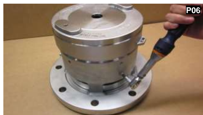
Use a 1/4" torque wrench or Allen key and loosen the three lift stops and remove.
