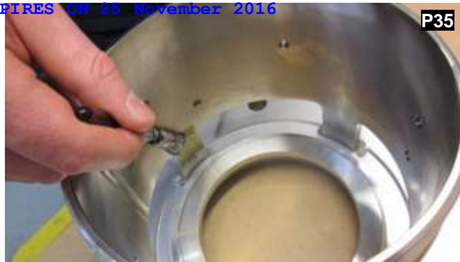
Apply Rocol on the 4 segments of the body tube. Lubricating assists smooth movement of the pressure plate.
