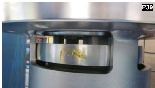
Continue lowering the ram until it has pushed the pressure plate free from the seal face, allowing the body to be lowered and screwed in to the cap. Ensure this gap exists throughout the entire circumference to avoid damaging the pressure plate o ring.
