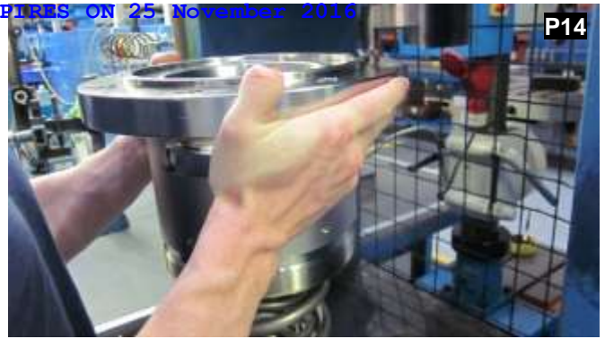
Once the spring is fully extended retract the ram completely allowing full access to the valve. Remove the main body. Inspect the main body for any damage.
