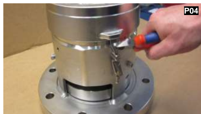
Cut the TIR wire and remove it by feeding it through the cable nipple.
