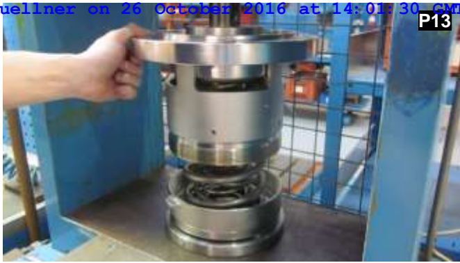
Slowly release the ram to allow it to take the load of the spring until the spring is released completely.
