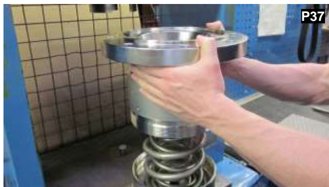
Slide the assembly towards the location pin on the press bed. Push the cap locator forward aligning the groove and the locating pin on the bottom of the press. This locates the assembly in the centre of the press and improves the alignment of the ram and the bore. Please refer P29.
