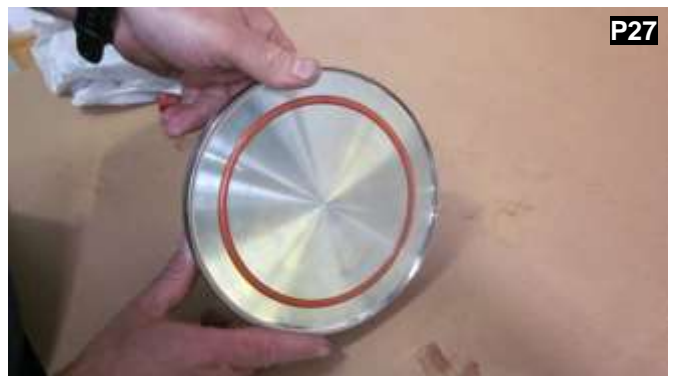
Check that the o ring is evenly clamped by the pressure plate.
