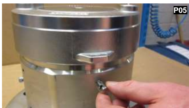
Remove the cable nipple.
