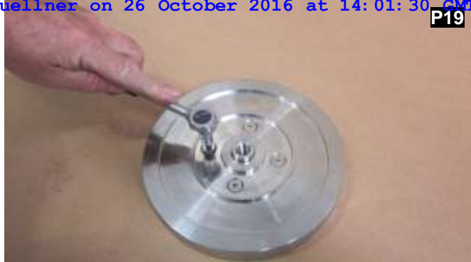
Place the part on a bench and remove the bolts by using a 5/32" torque wrench or Allen wrench.
