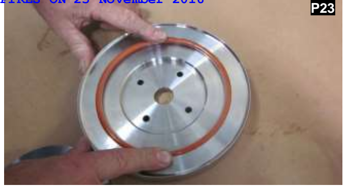
Locate the O ring in to the outer pressure plate as shown.
