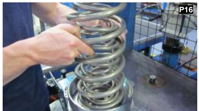
Remove the spring. Inspect the spring for any damage.
