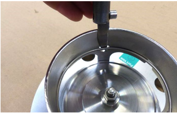
Step 19. Use a sharp-edged tool to release the retaining ring clip from the groove. Remove the clip.
