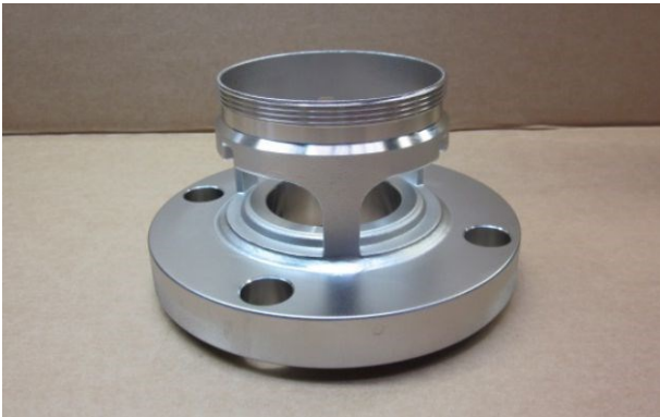
Step 21. Examine the body for signs of damage or corrosion. Look carefully at the pressure plate sealing face and the gasket sealing face. If there is damage, contact Fort Vale.
