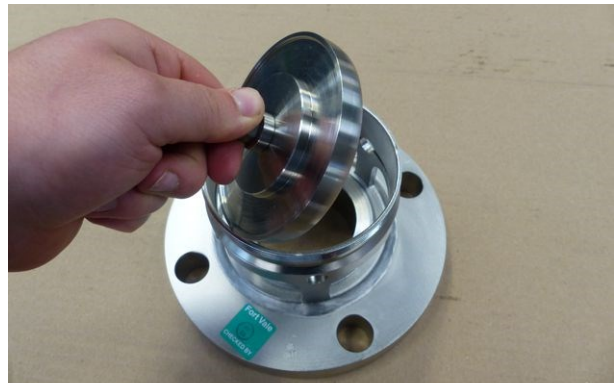
Step 20. Remove the pressure plate assembly.
