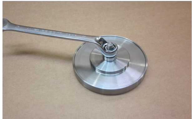
Step 22. DISASSEMBLE THE PRESSURE PLATE: Use a 1/2" (13mm) spanner to loosen the 5/16" UNF nut on the pressure plate assembly.
